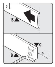
Slide outer rail (B) back and insert support plate (C) into outer rail (B). Support plate (C) must be installed at least 1" from desired length.
