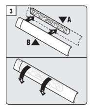
Attach aluminum rail (B) to mounting plate (A) by hooking from top and pushing until it clicks in place.
