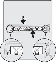
Determine a location for the organizer. Please note that the aluminum rail (B) extends past the mounting plate (A) so adequate clearance is necessary.
