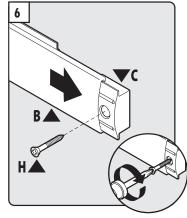
Fasten support plate (C) to mounting surface using screws (H) provided. Slide aluminum rail (B) back into place.
