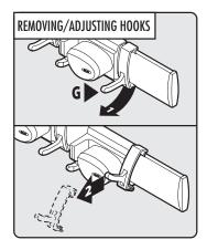
Lift hooks (G) from bottom to remove or adjust their positions. **Note:** Camlock™ holders (F) can only be removed by sliding them off of the rails.
