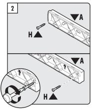
Line up mounting plate (A) with pencil marks. Arrows on mounting plate should be in up position. Fasten the mounting securely to wall using screws (H) provided.
