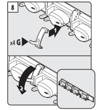
Hooks (G) attach from top of rail and snap into place.
