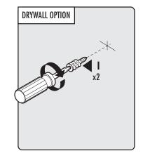
If not mounting directly into a stud, use drywall anchors (1). **TIP**: Put a starter hole in the wall for anchor to go in easily.
