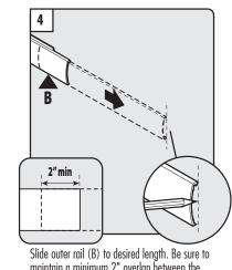
maintain a minimum 2" overlap between the inner and outer rails. Mark location on wall.
