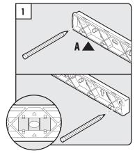
Mark hole on the left side of mounting plate (A). Level mounting plate using built-in level and mark hole on the right side of mounting plate (A).
